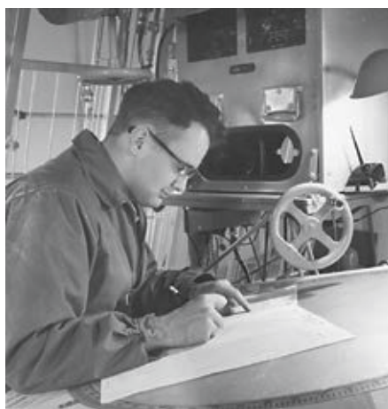
Newly installed "rawinsonde" upper air sounding equipment at St Paul, c1950. The dish antenna is visible behind the observer as a metal grid. As it rotates to track the balloon, the observer's seat and desk rotate around a common pivot in order to stay clear. The circular plotting board was used to graphically calculate the wind speed and direction. [NWS]
